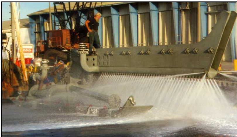
Figure E-3.5 Cable burial plow with jet pumps connected and running.
