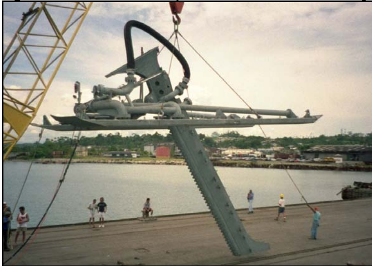
Figure E-3.5 Cable burial plow with jet pumps connected and running.
