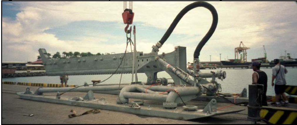
Figure E-3.3 - Cable burial plow with 5 meter blade fully retracted
